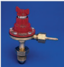
1465 - 0-2 bar (0-30 psi) Bijou variable regulator for propane with 3/8in BSP-LH male union outlet and 4.8mm hose end supplied (No 1021) 1465X - 0-1 bar (0-1 psi) Bijou variable regulator for propane with 3/8in BSP-LH male union outlet and 4.8mm hose end supplied (No 1021)
