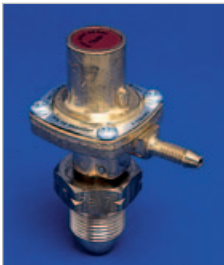
4041 - 4 bar pre-set brazing regulator for propane with integral 4.8mm hose outlet
