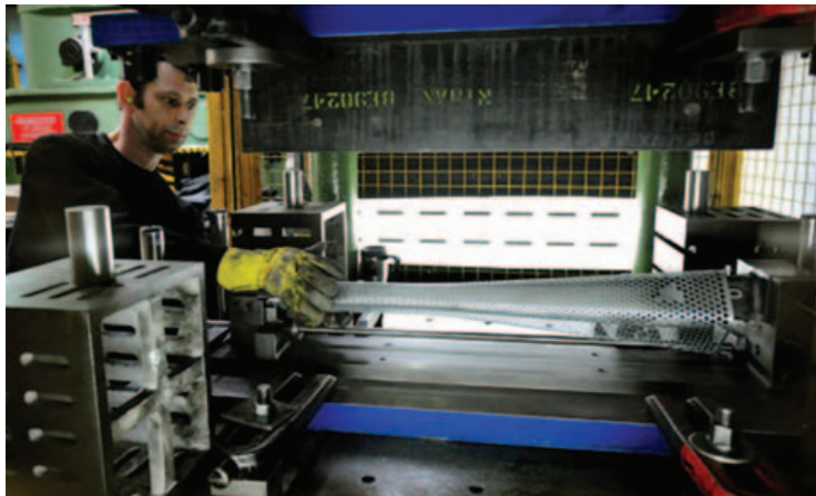
An Olympic Torch being pressed at the Premier Group factory in Coventry © Rui Vieira/PA Wire Ref #: PA.13368430
